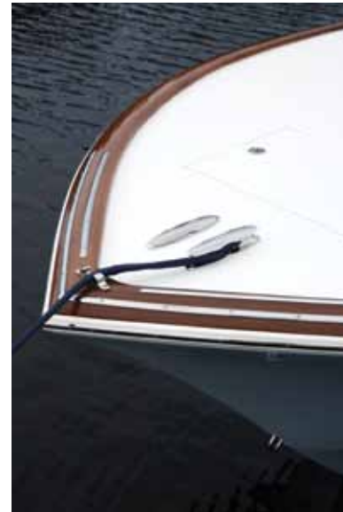
Thick Mahogany toe rail with welded stainless steel rub rails.
